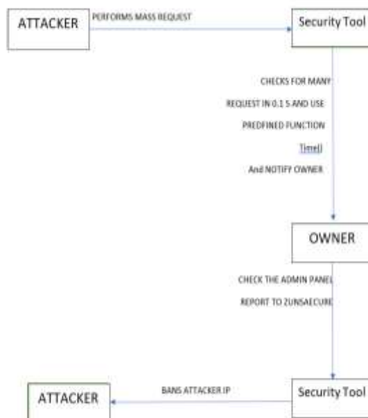
FIGURE 3: Detailed Block Diagram
